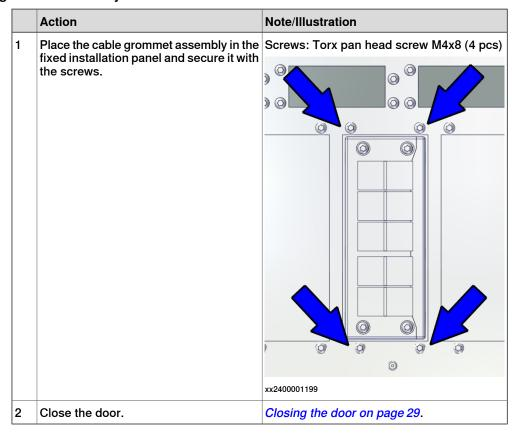
5.1.5 Replacing the process cable gland
